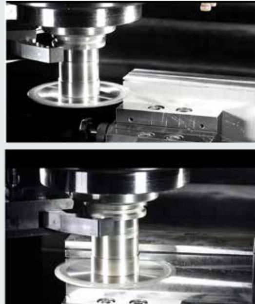
TCT saw blade for deep saw cuts, slotting or milling.
