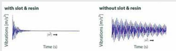
Noise reduction due laser slots with resin
