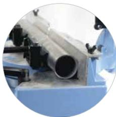
Incl. Fixing set „K“ for pipes
