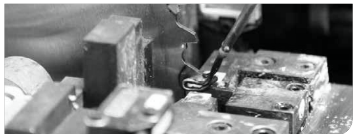
soldering the carbide teeth
