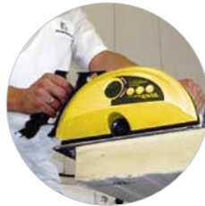
Cuts sheet metal up to 3/8" (10 mm) and sandwich panels and profiles with a cutting depth of up to 3 3/4" (82 mm)
